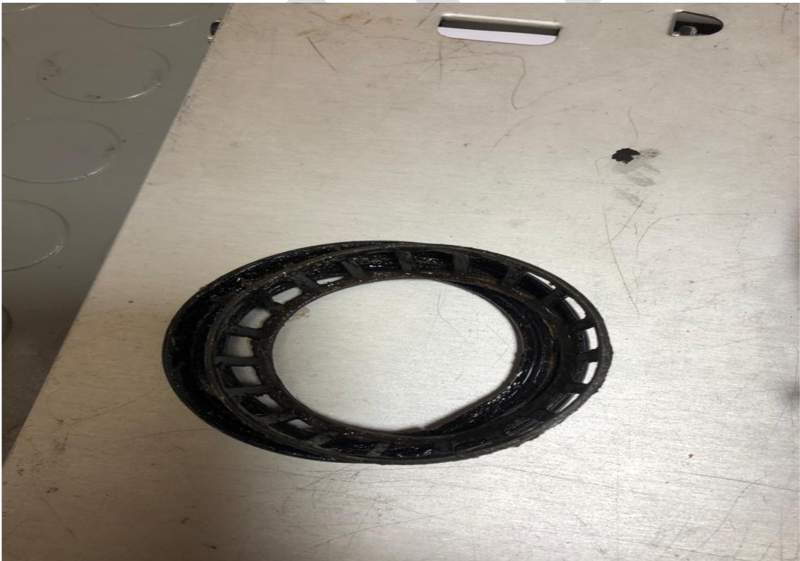
Resim-7: Nose Wheel Bearing Hasarı
