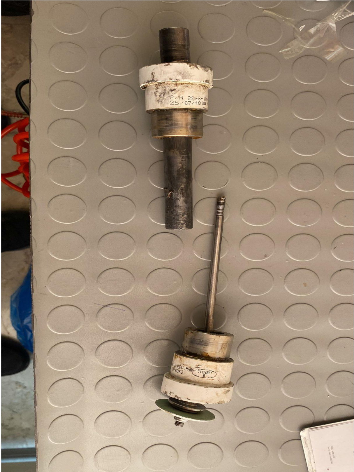
Resim-4: NLG Control Bushing, Internal Bushing Hasarı
