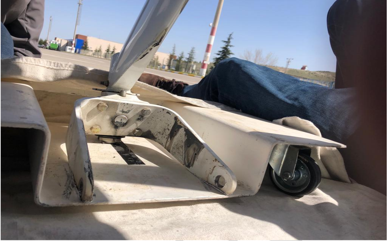
Resim-3: NLG Threaded Shaft Hasarı
